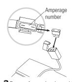
**3** Remove fuse and replace with a new one of equal amperage. **Note:** Amperage is located on top of fuse. Fuse must be replaced with one of equal amperage.
